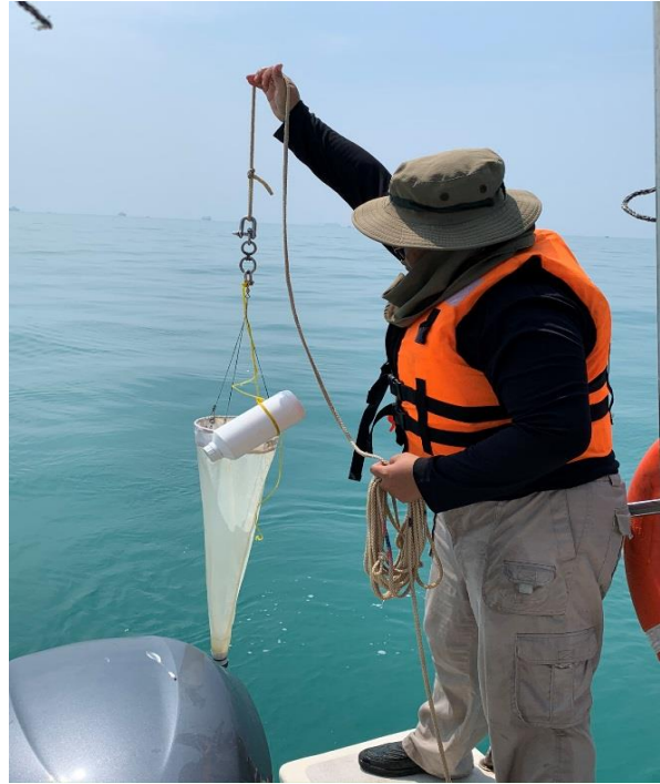
Plankton sampling utilising a plankton net
